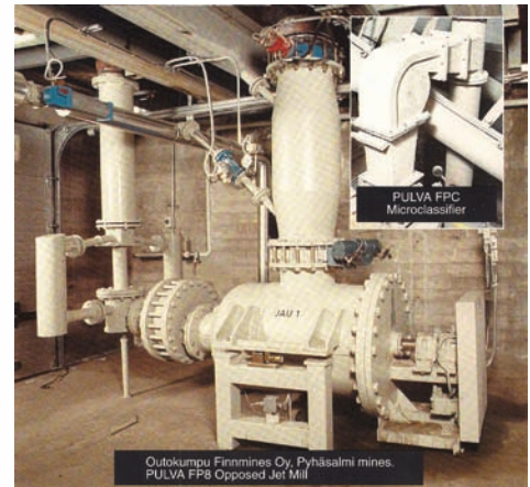
Opposed Jet Mill with mechanical classifier in Pyhäsalmi Mine
