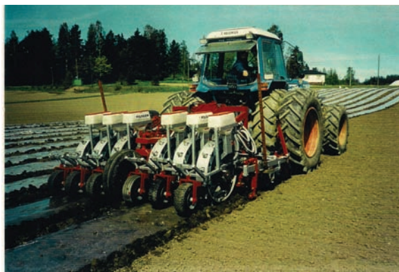
The automatic sowing machine prepares the bench, fixes biofilm on top of it, punches holes through it and sows the seeds through the small holes.
