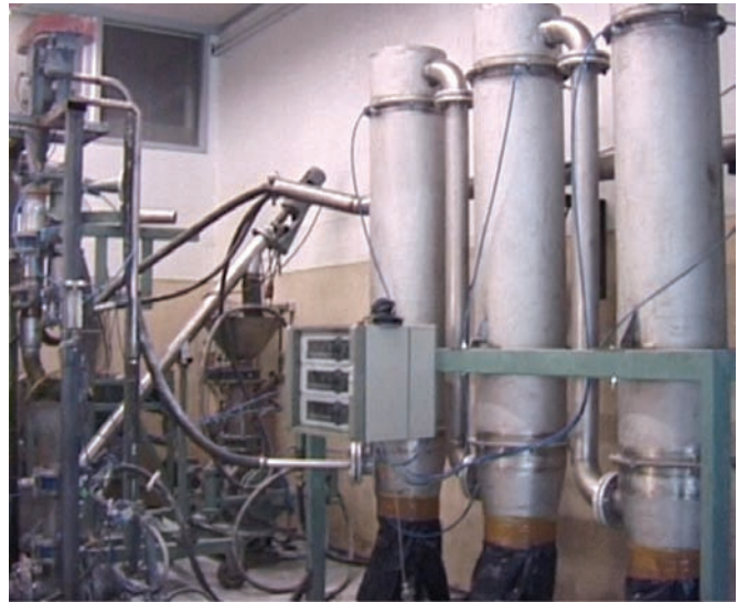
Opposed Jet Mill and Ion Particle Classifier separate minerals in the pilot facility (One milligram of Platinum from 1000 kg of iron ore).
