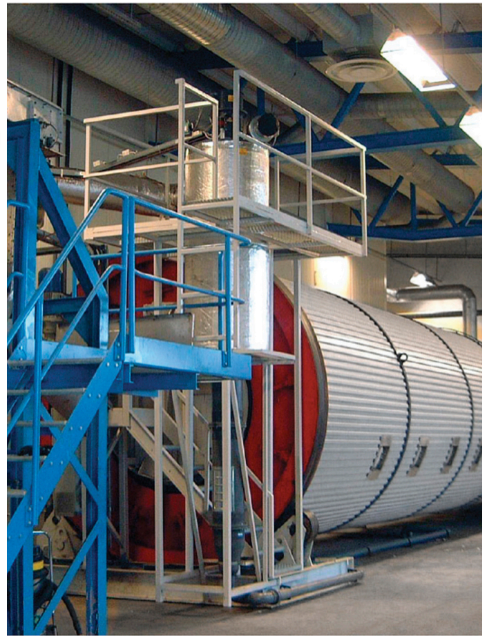
Every bio-oxidizer is equipped with the air cleaner (30 000 m 3 /h).
