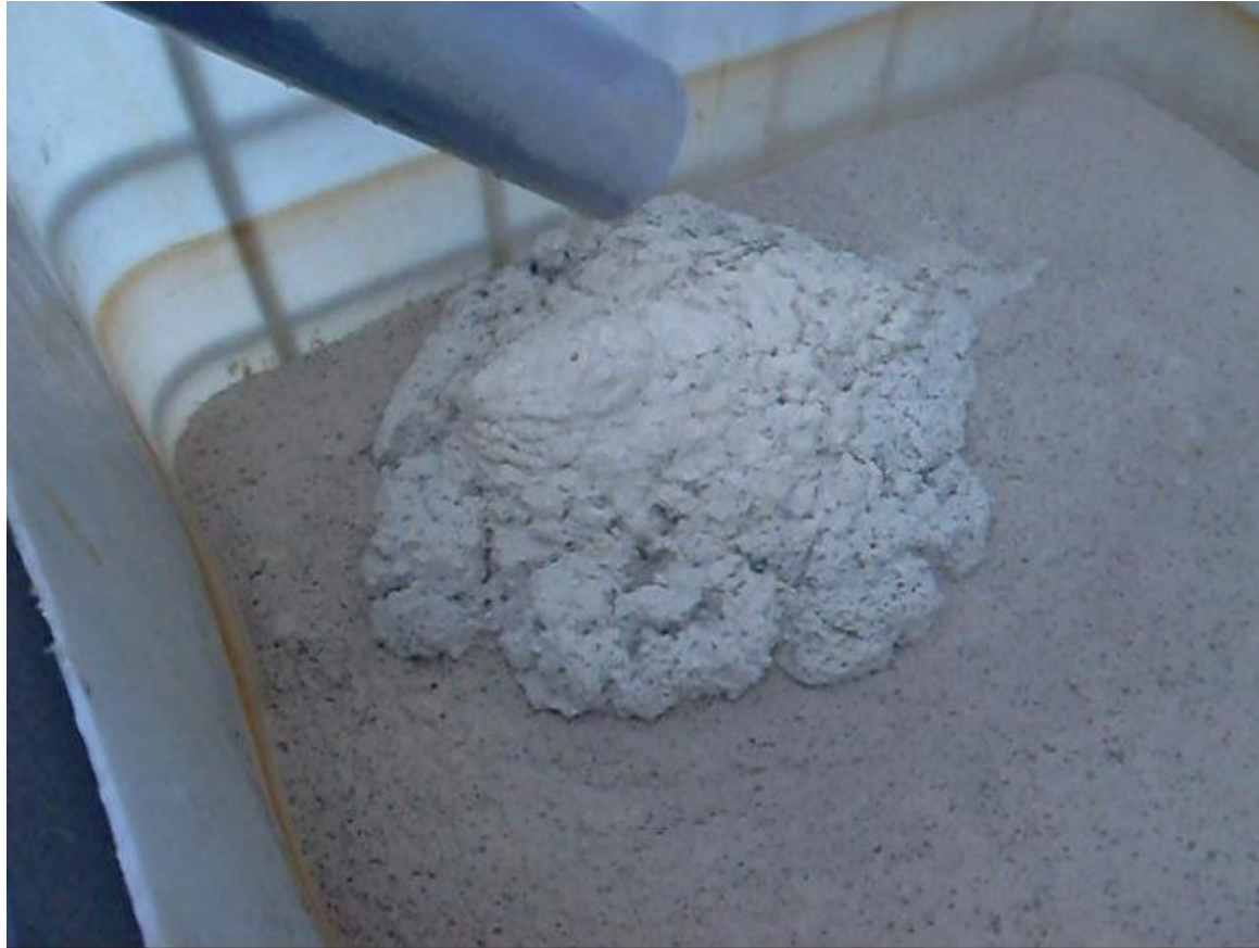
Picture 10: Video clip: The separated floc from the tower drops to the decanter for further dewatering where it will dry by itself up to the dry matter of 90 % .
