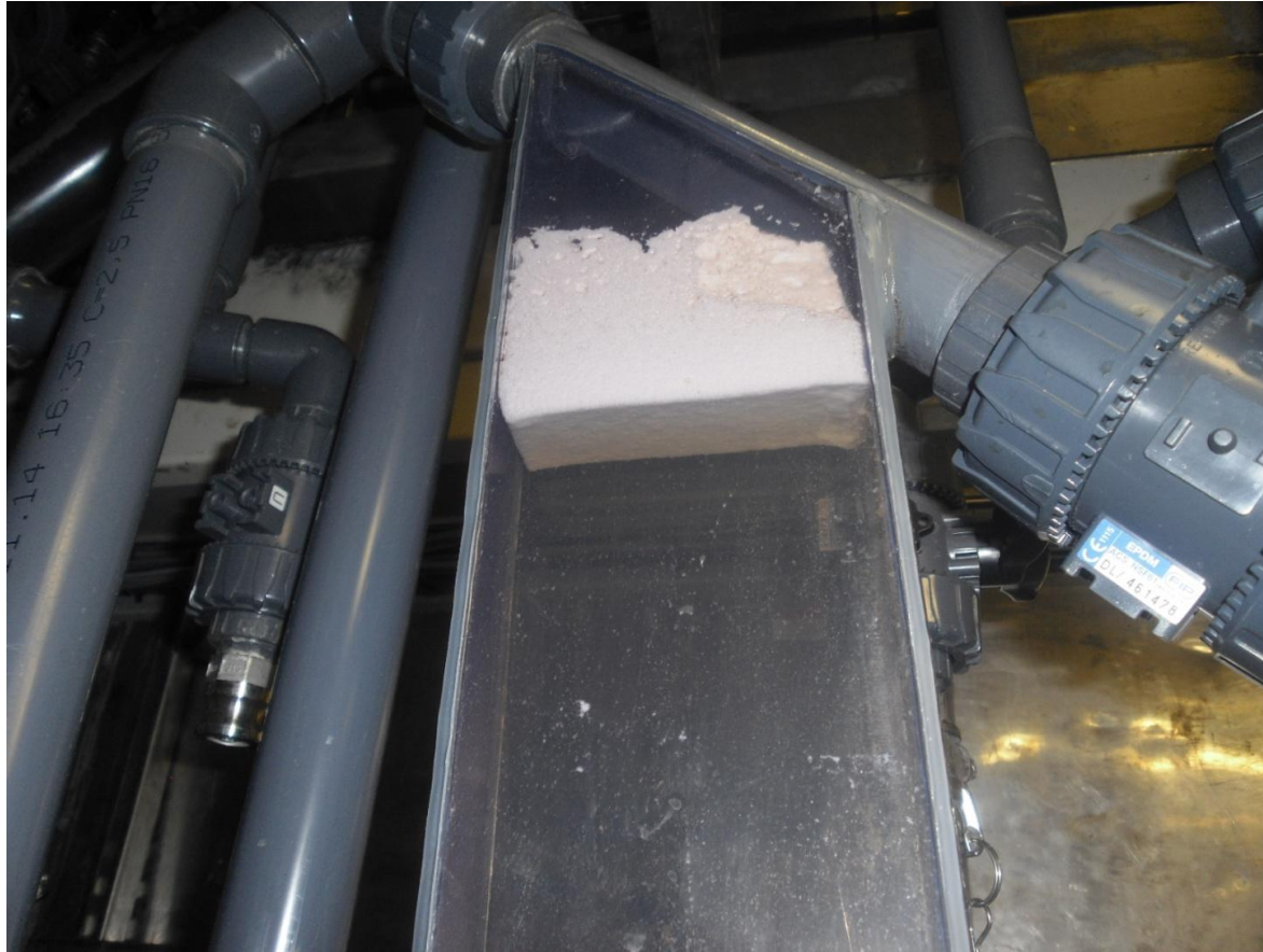
Picture 4: The stable floc with impurities is distinctly floating on the surface of the purified water as seen in the see through glass when the preliminary test with the first cascaded cell was completed.
