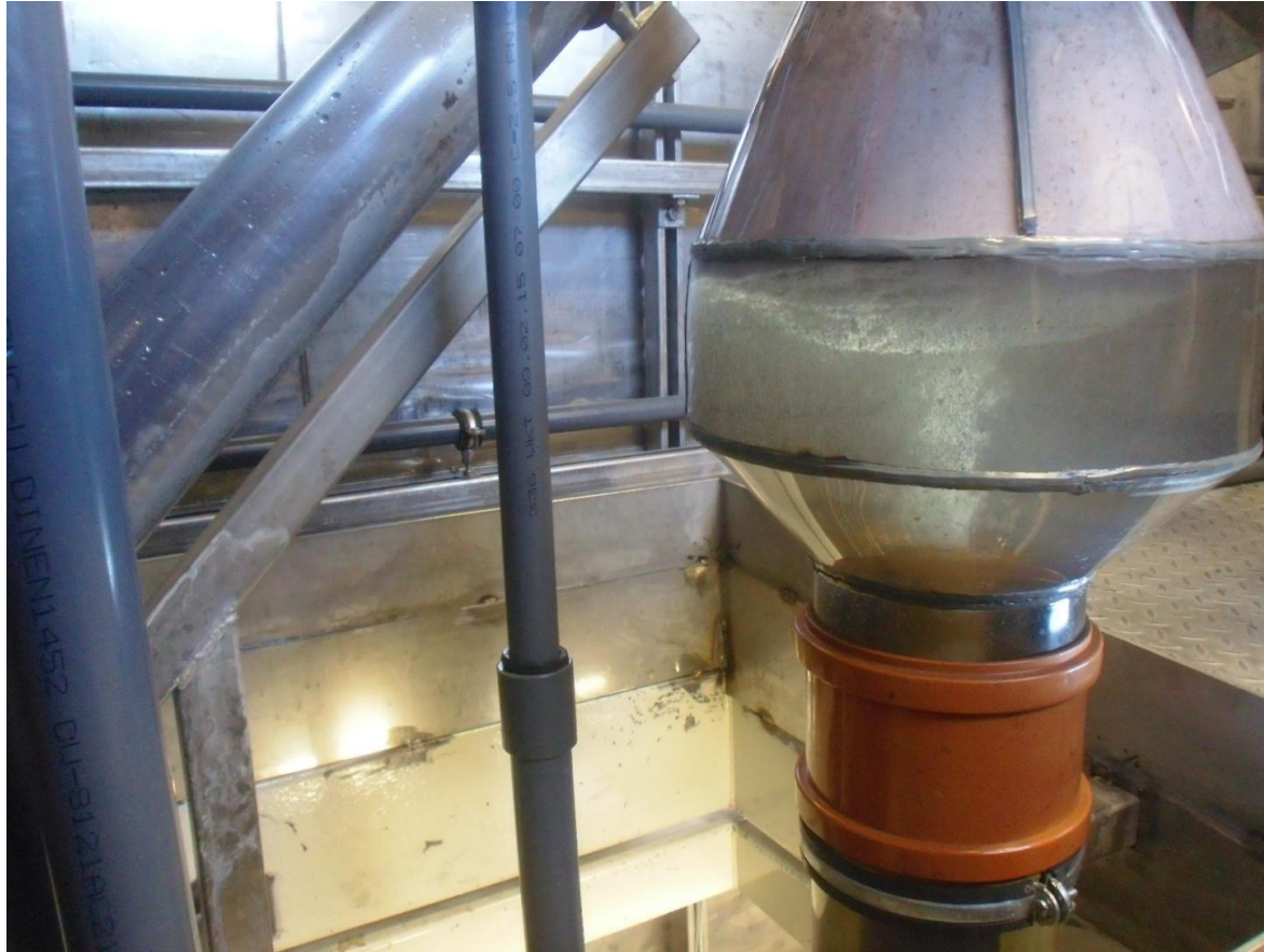
Picture 7: The Purified Water starts to separate from gas containing solid floc in the expansion part of the tower, when leachate leaves the MUST cell and enters into the floc separation tower .
