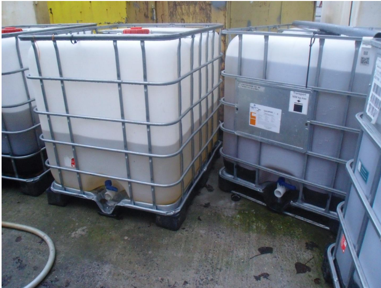
Picture 2: 6000 liters of leachate water from IMOG was brought to the pilot site of MUST for optimizing the purification and reduction of COD -value to less than 200 mg/l.
