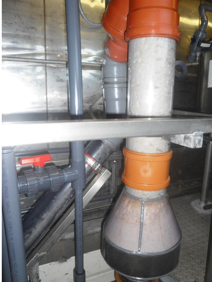
Picture 8: The foamy, white colored floc is dewatered when it rises up to the top of the tower. From the open top of the tower the floc will enter into the dropping tube without mechanical devices. The purified water flows downwards from the sharp “rack level” in the expansion part of the tower.
