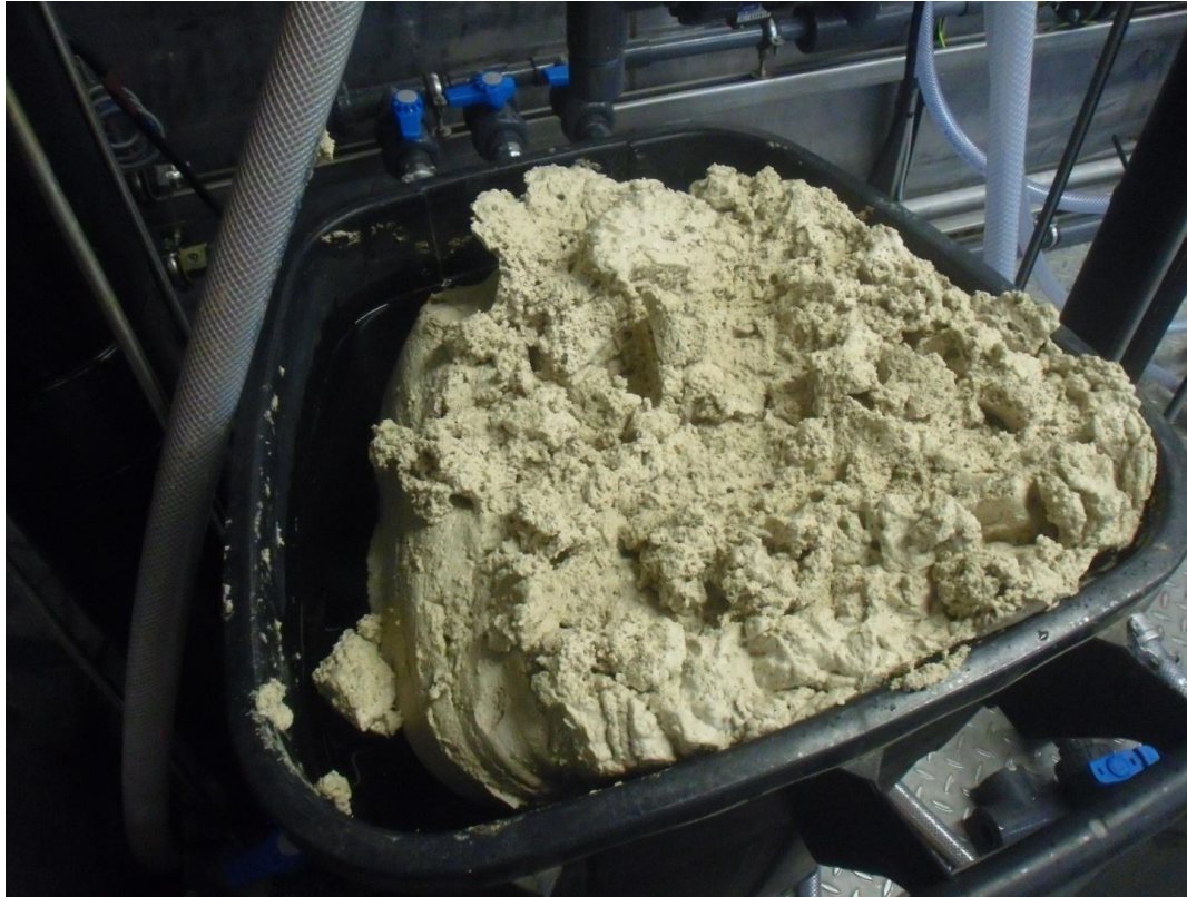
Picture 5: The floc, which is floating on the purified water in the basket, was settling from the leachate after it was pumped through the first cascaded cell and was collected from the see through glass, in the preliminary test, before introducing the flocculating mixture into the floc separation tower.
